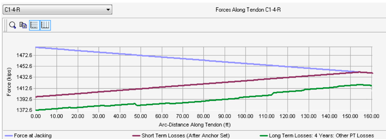
C1-4-R (Tendon B) Force Profile after Four Years
